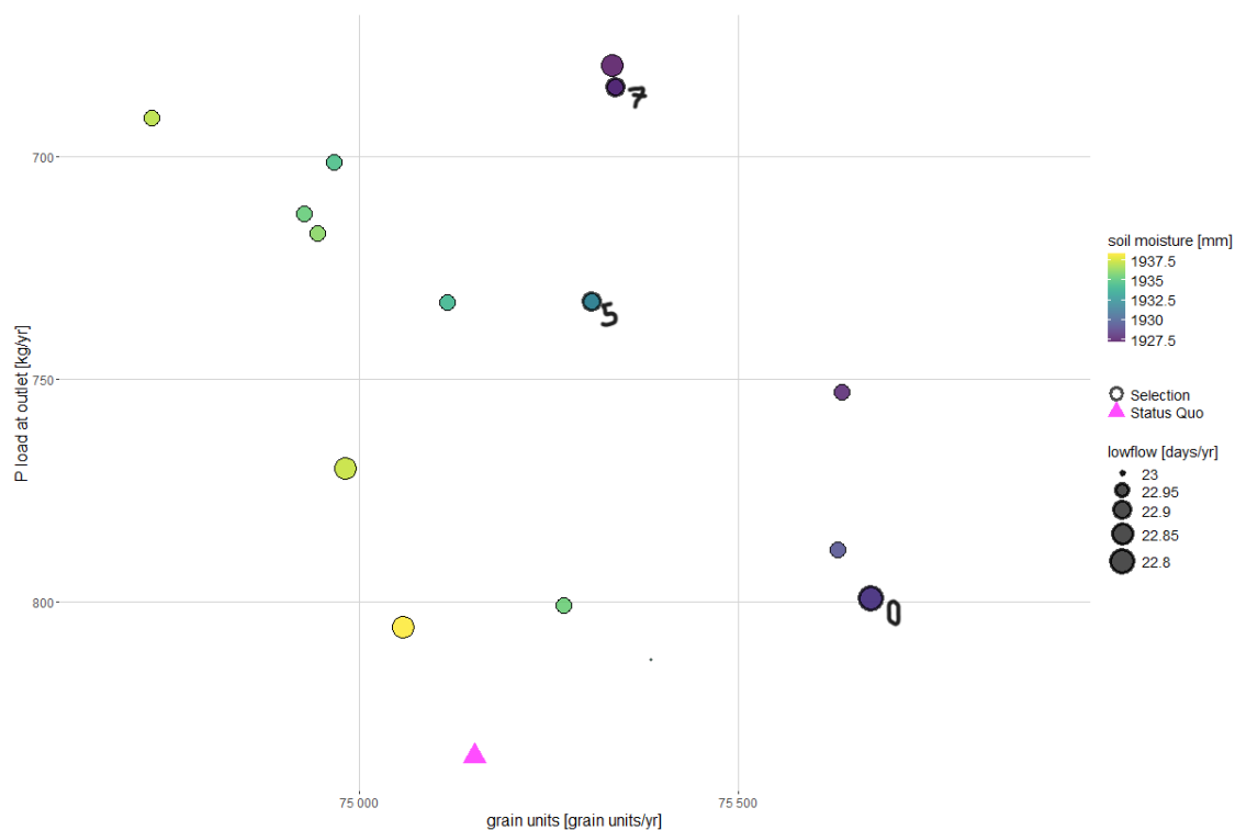
Figure A7: Scatter plot of the Pareto optima remaining after clustering. The three largest clusters (0, 5, 7) are marked in bold. Example from case study 2 Petite Glâne.
