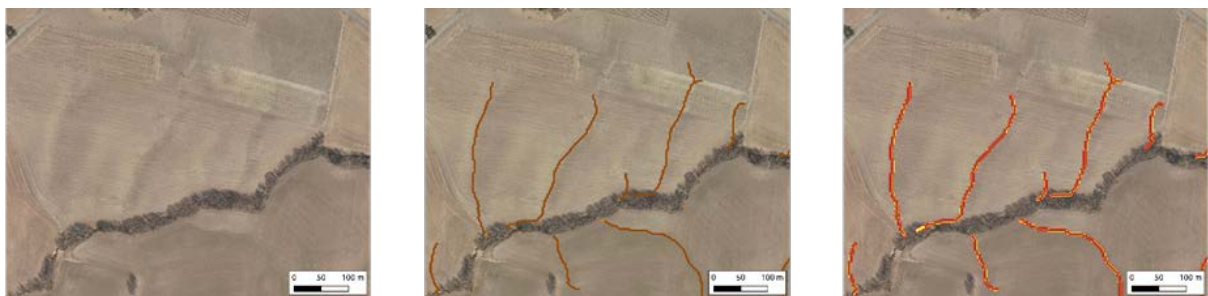
Fig. A10.18 Placement of grassed waterways: terrain > gully erosion risk > grassed waterways (6 m width). Source: Robert Barneveld (NIBIO)
