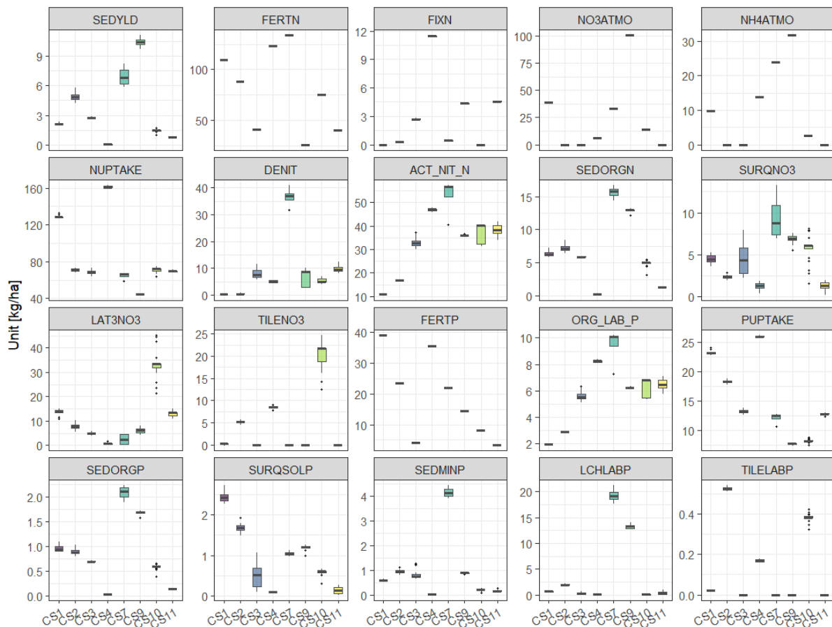
Figure 3.4: Simulated values of selected basin-averaged sediment and nutrient outputs for the baseline period for all CS. Note that the unit for 'sedyld' is [t/ha]. Full description of indicators and their units provided in Annex 16.
