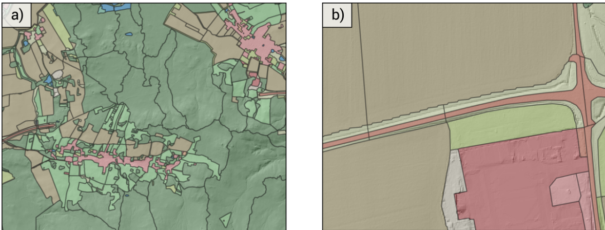
Figure 2.6: Details of a land object layer. a) shows the division of a large forest (dark green area) into smaller units based on local catchments. b) shows the splitting of long objects e.g. roads into shorter segments based on borders of neighbouring units.
