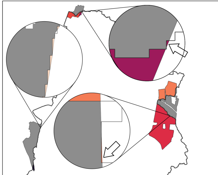
Figure 2.10: Identification of MULTIPOLYGON issues for an example land layer after the intersection with the basin boundary. The details point to the small fragments which were generated during the intersection and which have to be removed.
